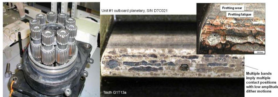
RSB actuator planetary gear corrosion damage.
