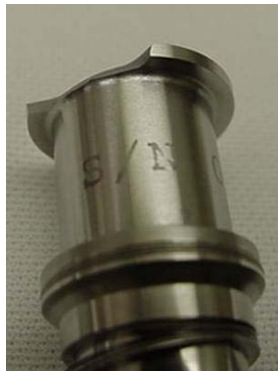
Figure 20: STS-126 broken FCV poppet
