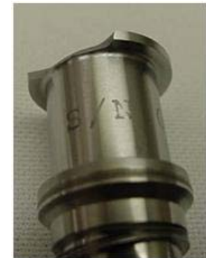
STS-126 broken FCV poppet
